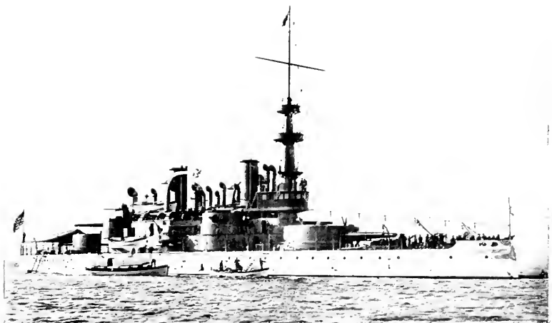
U. S. BATTLE SHIP INDIANA, 10,288 TONS DISPLACEMENT. Length 348 ft., beam 69.3, draft 24. Built by Wm. Cramp & Sons, Phila., Pa. Copyright 1896, by J. S. Johnston, N. Y.
